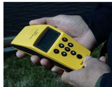
Kinematic data collection is a collection technique where data is collected continuously along a pathway (in this case along the waterway). GPS units are programmed to collect information at a rate sufficient to compute a position anywhere along the course. Features are collected at a rate of one observation every five seconds. Land use, bank condition, and linear shoreline structures are collected using this technique.
