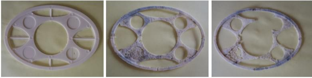
Time sequence of biodegradation of PHA panel (prior to use, six months, 12 months).
