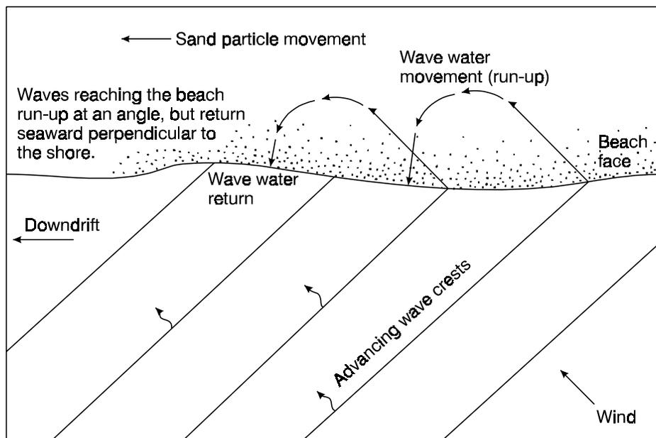
By moving each grain of sand slowly along the shoreline in small continuous arcs, the alongshore currents are capable of transporting a considerable amount of sediments over time. It is this sand transport which fills the groins constructed along the shoreline, builds sand bars, and contributes to the shrinking or expansion of existing beaches.
