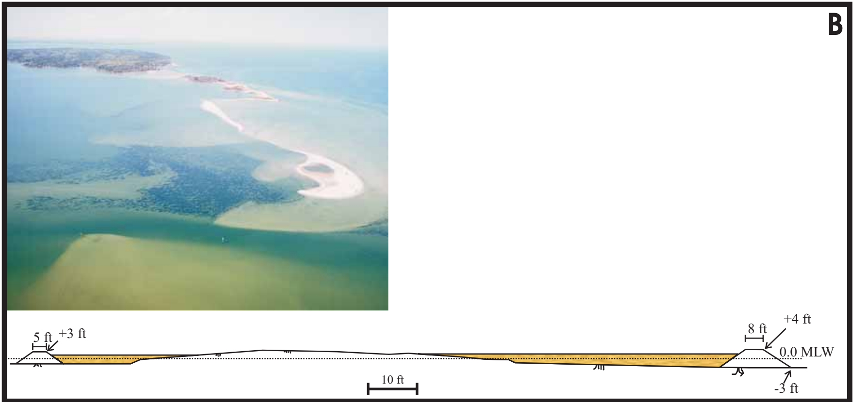
Figure 6-9. Typical cross-sections of breakwaters and beach fill for A) for the Bay coast of Mathews and B) for Rigby Island which requires protection on both the Bay side and lee side in Milford Haven.
