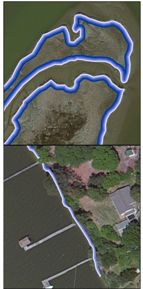
Depiction of 1-m intervals along marsh edge used in mussel surveys and areal estimates of marsh habitat
